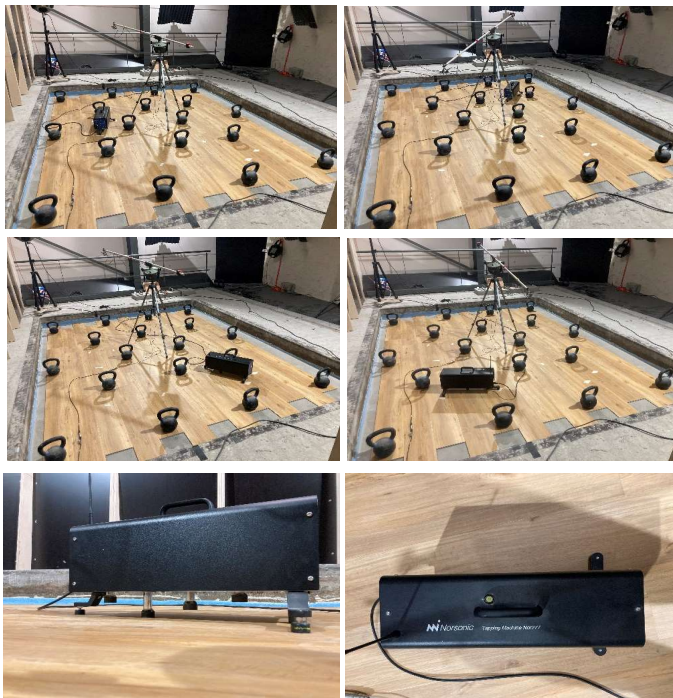
Photos of the four tapping machine positions on the tested floorcovering:
